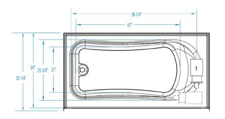
AFR allows for above the floor installation of waste, overflow and drainage. This unit is standard as AFR. Optional cut skirt available.
