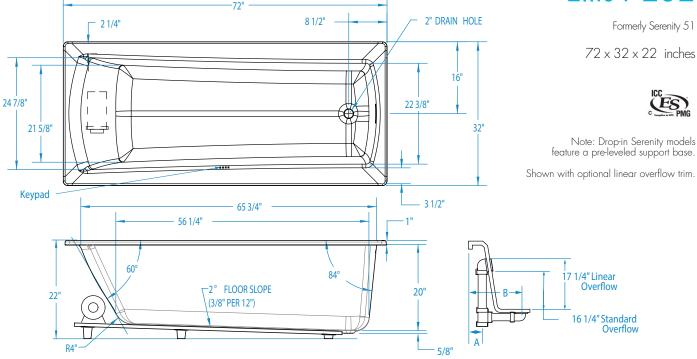
FEATURES Dimensional Tolerance ± 3/8". Dimensions needed for site preparation should be measured from the unit. Manufacturer assumes no responsibility for preparatory work.
