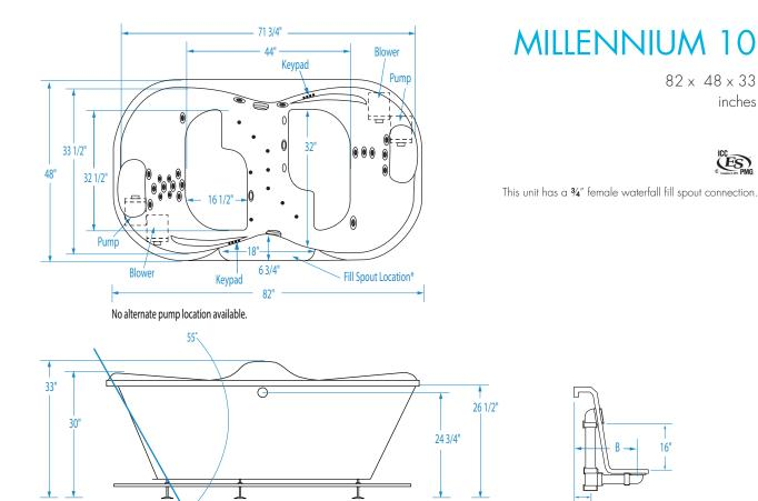
FEATURES Dimensional Tolerance ± 3/8". Dimensions needed for site preparation should be measured from the unit. Aquatic assumes no responsibility for preparatory work.
