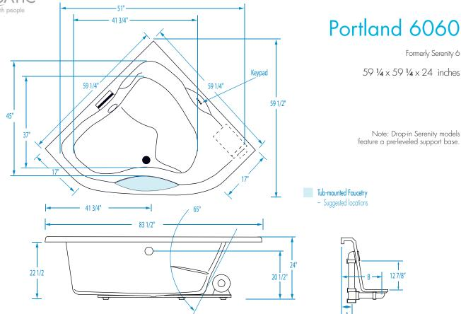
FEATURES Dimensional Tolerance ± 3/8". Dimensions needed for site preparation should be measured from the unit. Manufacturer assumes no responsibility for preparatory work.
